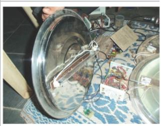
**UV filter for drinking water:** The lid for a 20 litre steel container is fitted with a UV lamp which can run either on 220V AC or 15V DC from solar power.
